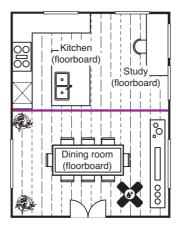
If there was damage to the flooring at the spot marked 'X' in the dining room, we would only repair or replace the flooring within this functional area up to the purple line. In this scenario, we may need to introduce a floor trim along the purple line.
