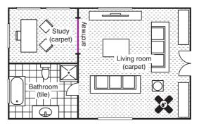
If there was damage to the flooring at the spot marked 'X' in the living room, we would only repair or replace the flooring within this functional area. In this scenario, we may need to introduce a floor trim between the study and living room as per the purple line, since the damage is contained within the living room alone.
